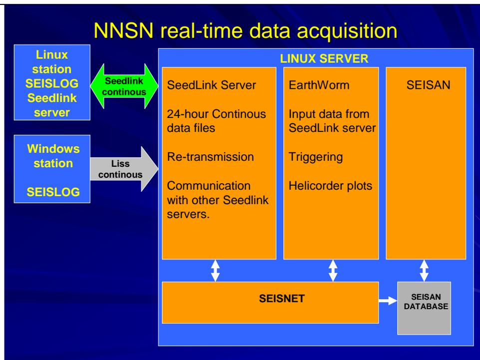
Figure 2. Diagram showing the NNSN real time data flow.
